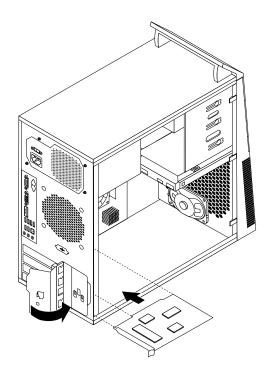
Figure 13. Installing a PCI card
